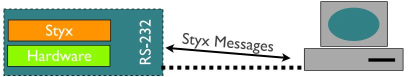
This device can now access network<br/>protocol stack, process control, displayReal world example: Styx on Lego Rcx<br/>Brick (Hitachi H8 microcontroller, 32K<br/>RAM, 16K ROM)
